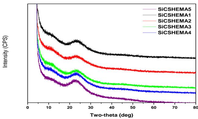
Fig.1 XRD patterns of synthesized hybrid nanocomposites
