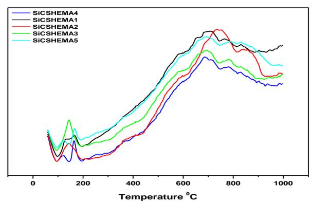
Fig. 3 DTA curves of synthesized hybrid nanocomposites
