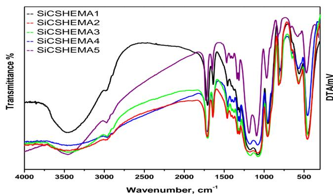
Fig. 2 FTIR spectra of synthesized modified silica nanocomposites
