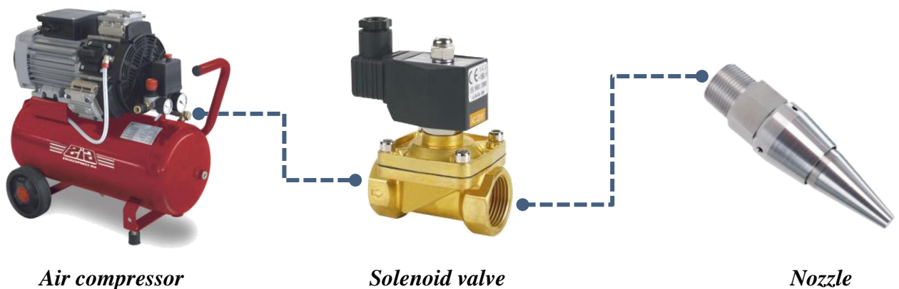
Fig. 1: Dust blowing system
